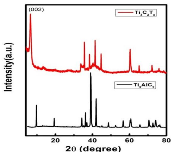
**Figure 1.** X-ray diffraction spectra of Ti<sub>3</sub>AlC<sub>2</sub> (MAX phase) and Ti<sub>3</sub>C<sub>2</sub>T<sub>x</sub> (MXene).
