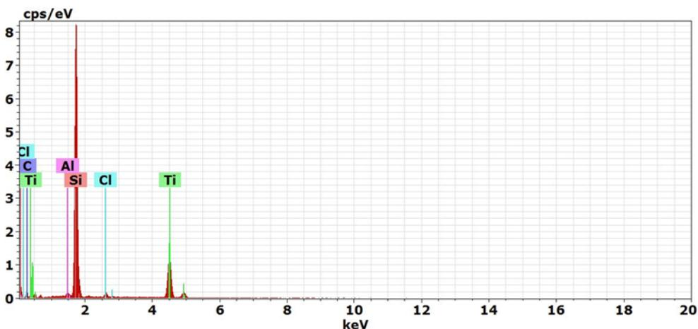
**Figure 3.** Typical EDX spectra of Ti<sub>3</sub>C<sub>2</sub>T<sub>x</sub> after the selective etching of aluminium layers from the MAX Phase.
