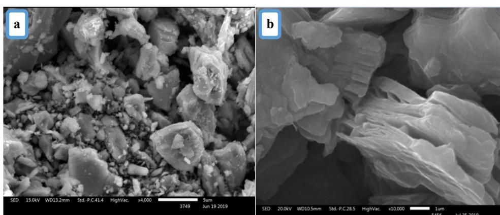
**Figure 2.** (a) Represents the SEM pictograph of Ti<sub>3</sub>AlC<sub>2</sub> (MAX Phase) and (b) represents the exfoliated accordion type morphology of stacked layers of Ti<sub>3</sub>C<sub>2</sub>T<sub>x</sub> (MXene) flakes.
