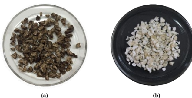
Figure 4. Photographs of the synthesized dried cellulose-based hydrogels: (a) CPC-hydrogel from CPC, and (b) CRC-hydrogel from CRC.
