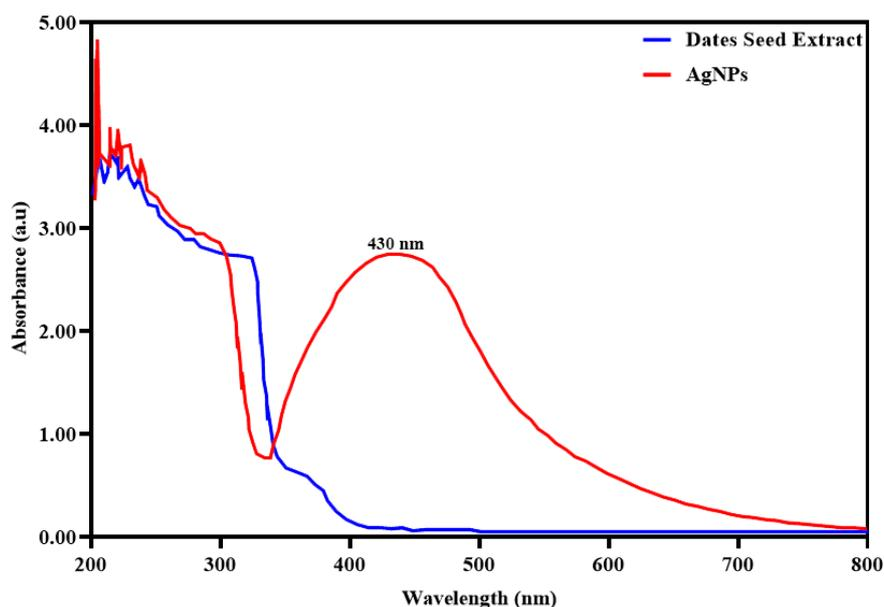
**Figure 1.** UV-Vis spectra of silver nanoparticles synthesized using Egyptian date palm seed extract.
